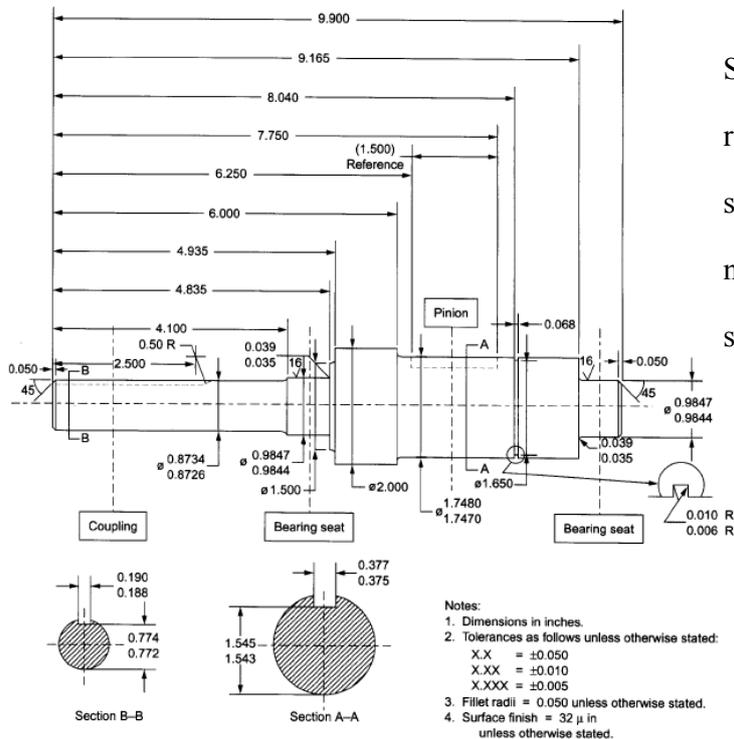
Significant detail is required to completely specify the geometry needed to fabricate a shaft.
