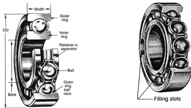
Figure 9. Ball bearing components
