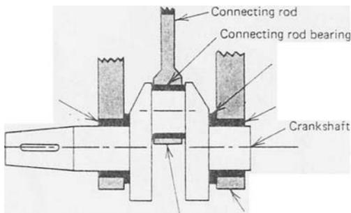
Figure 11. Crankshaft and plain bearing
