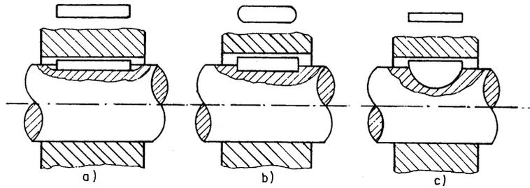
Figure 4. Types of keys, a and b : rectangular parallel keys, c: woodruff, [2]
