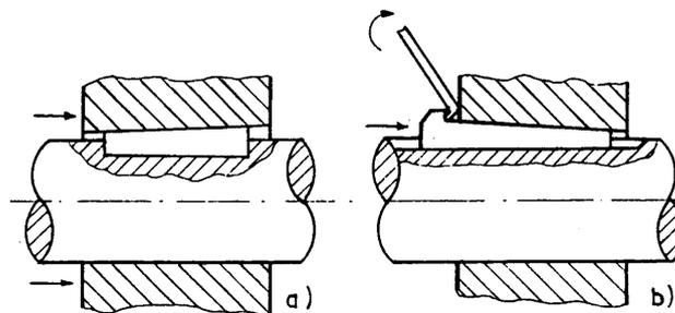
Figure 5. a: Tapered keys (friction will help transmit torque and provide resistance to axial motion of the hub relative to the shaft),
