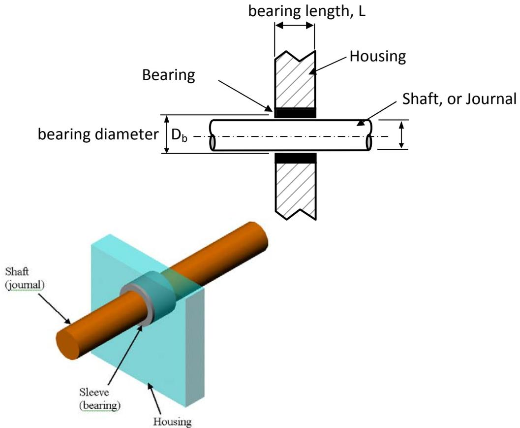
Sliding bearings require direct sliding of the load-carrying member on its support, as distinguished from rolling-element bearings, where balls or rollers are interposed between the sliding surfaces.
