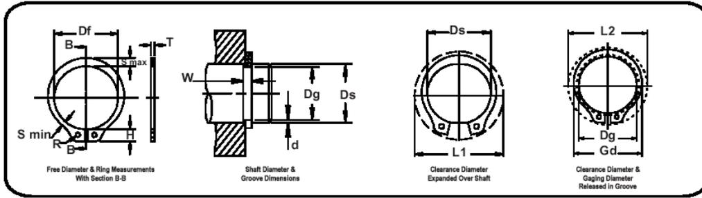
Figure 8. Snap rings which provide a removable shoulder to lock the components on shafts.
